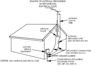
Electrical Code, ANSI/NFPA No. 70, provides information with respect to proper grounding of the mast and supporting structure, grounding of the lead-in wire to an antenna discharge unit, size of grounding conductors, location of antenna-discharge unit, connection to grounding electrodes, and requirements for the grounding electrode. See Figure 1.
